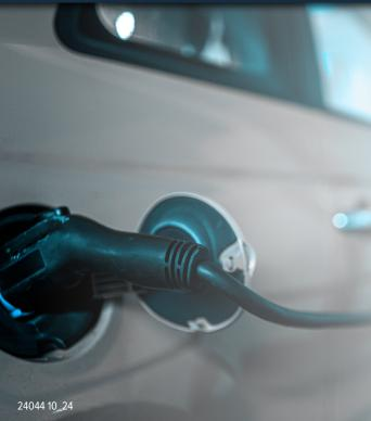
A Level 2 electric vehicle charger can cut your charging time in half or more, with a full charge in as little as four hours.
