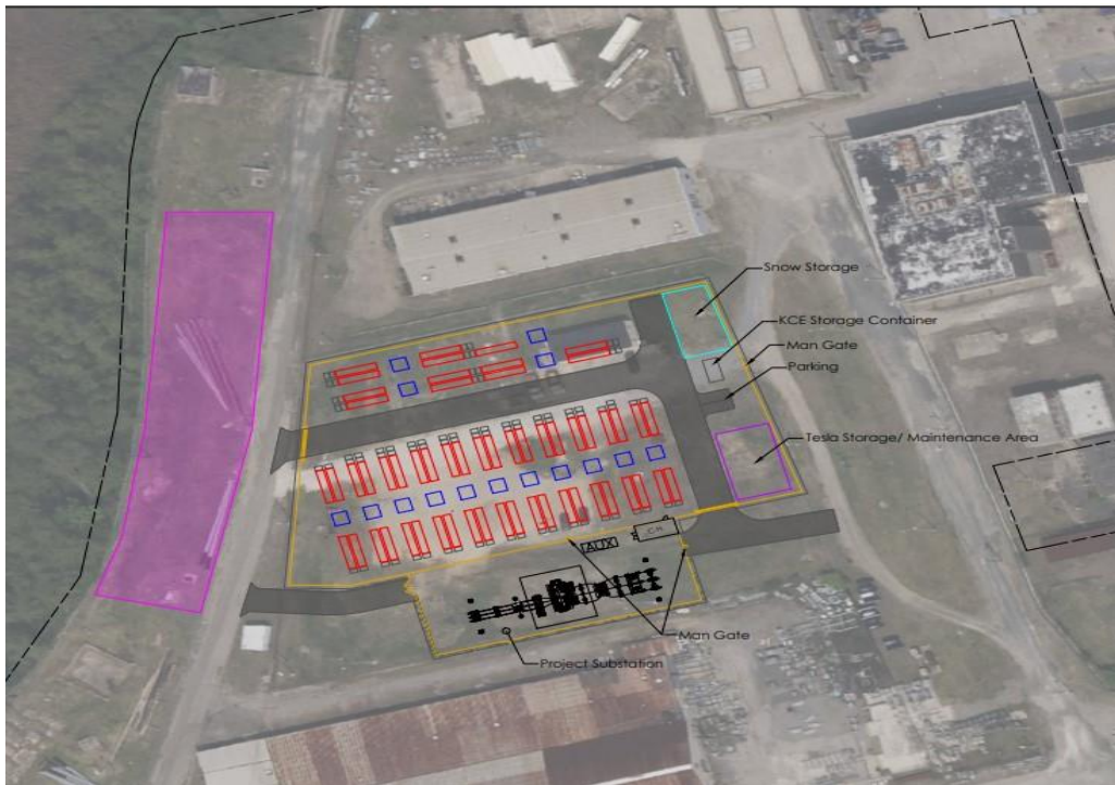
Figure 1. BESS Facility Overview
