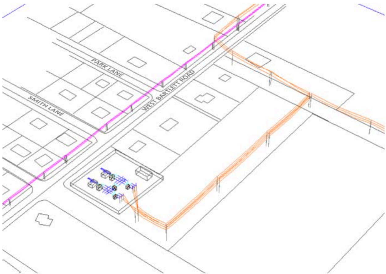
Figure 4. Overview of the three-dimensional SUBCALC model used to calculate magnetic-field profiles in the vicinity of the proposed West Bartlett Substation for the average and peak loading cases in 2017.
