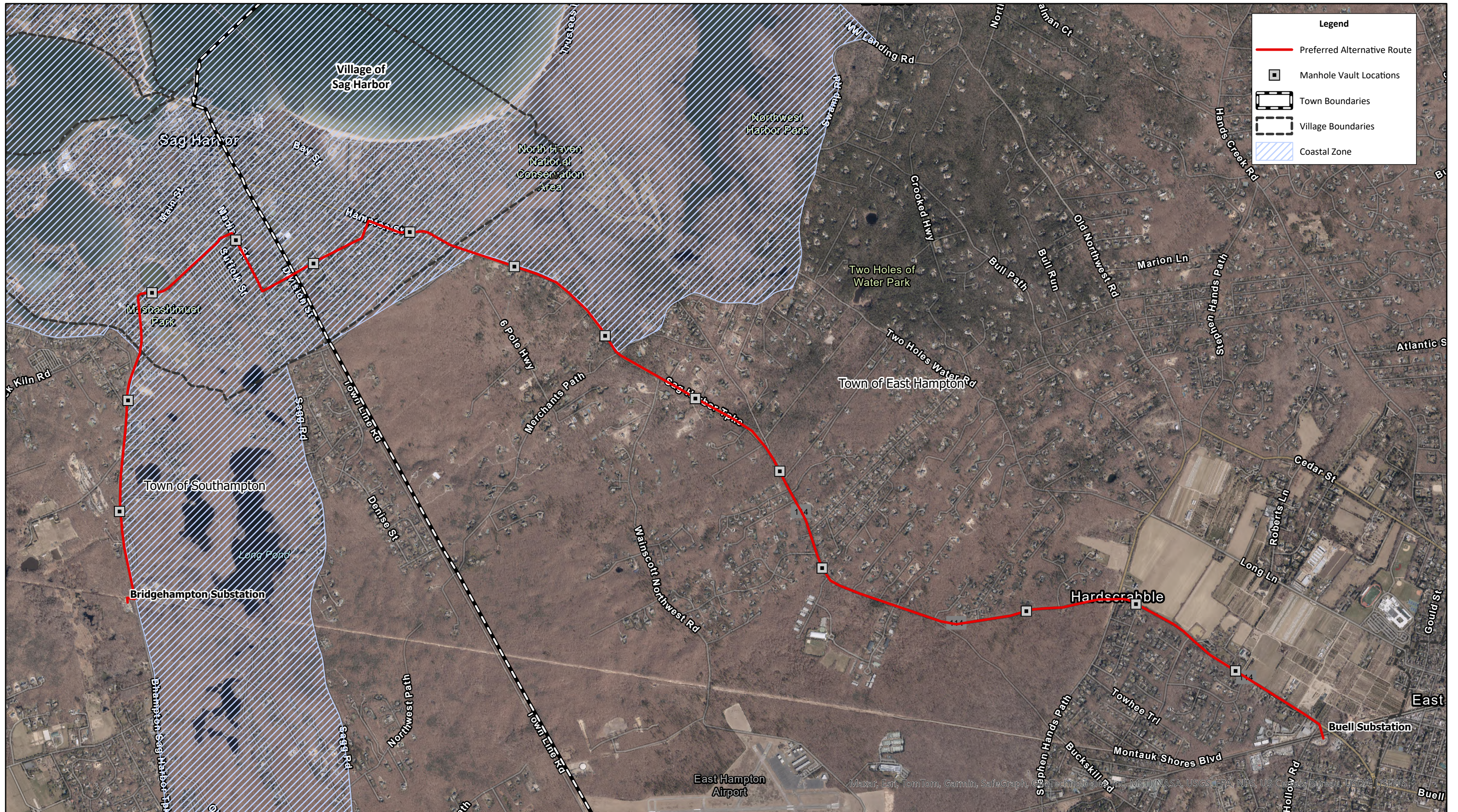
FIGURE 2 COASTAL ZONE AREA MAP BRIDGEHAMPTON TO BUELL NEW 69KV UNDERGROUND TRANSMISSION CABLE
