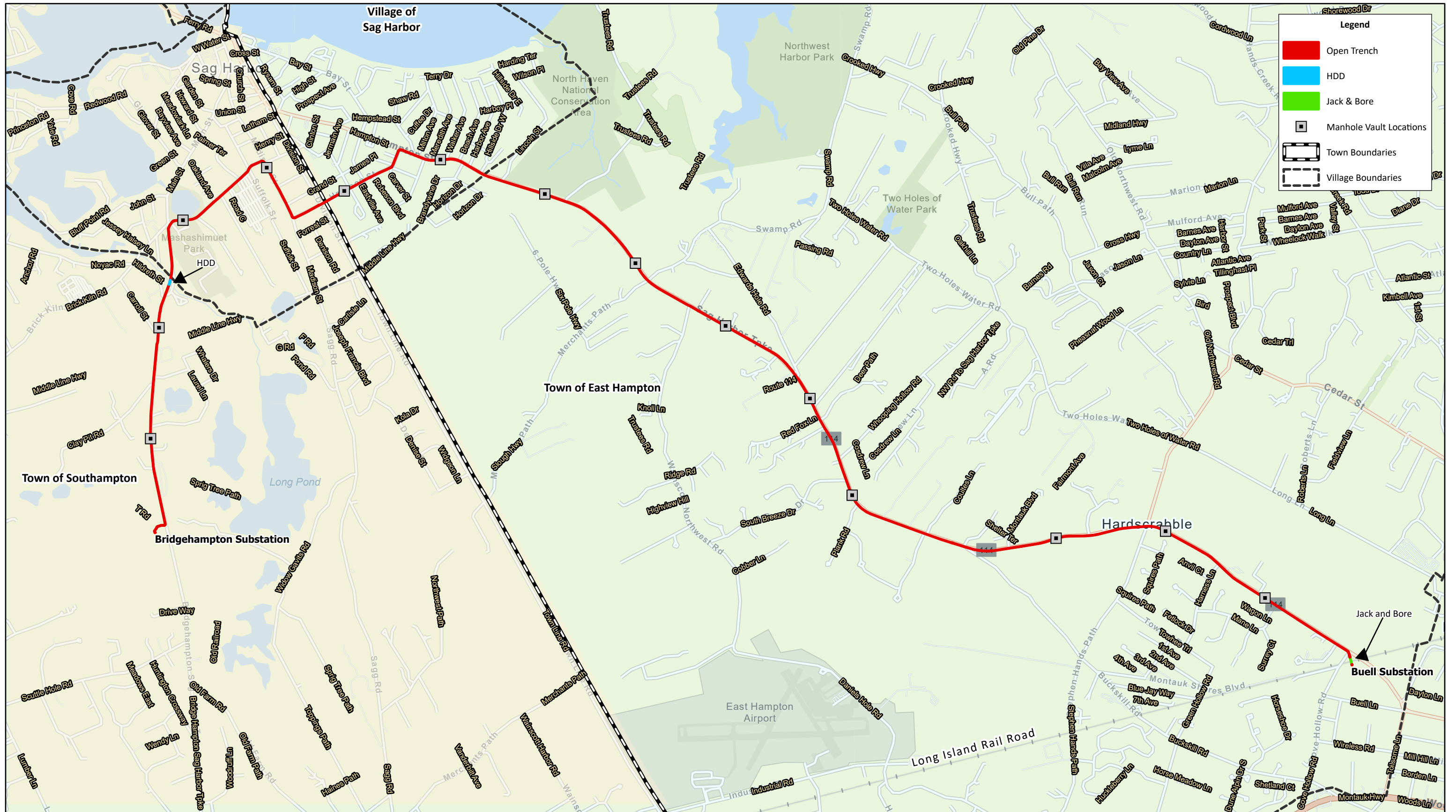
FIGURE 1 PREFERRED ALTERNATIVE ROUTE MAP BRIDGEHAMPTON TO BUELL NEW 69KV UNDERGROUND TRANSMISSION CABLE Sources: NYS Orthoimagery, 2023; Suffolk County GIS, 2024
