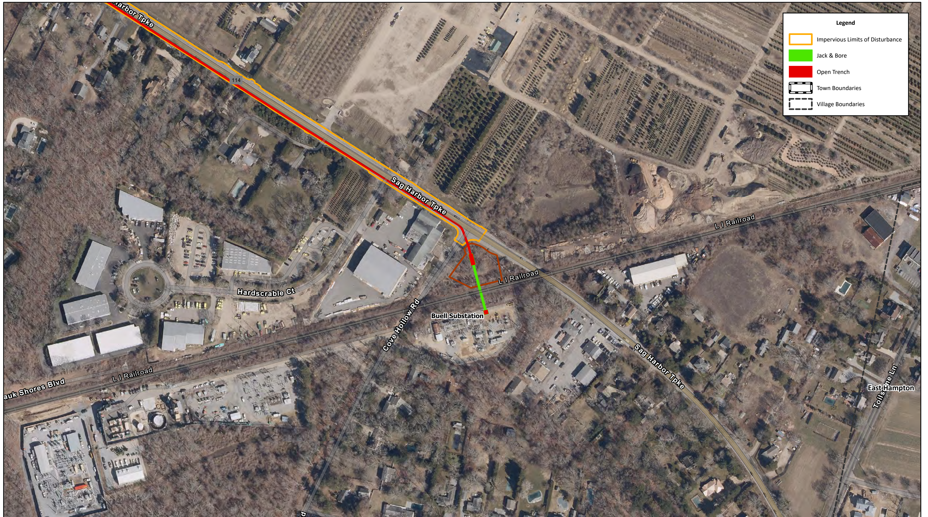
FIGURE 2-16 AERIAL MAP BRIDGEHAMPTON TO BUELL NEW 69KV UNDERGROUND TRANSMISSION CABLE Sources: NYS Orthoimagery, 2020; Suffolk County GIS, 2024
