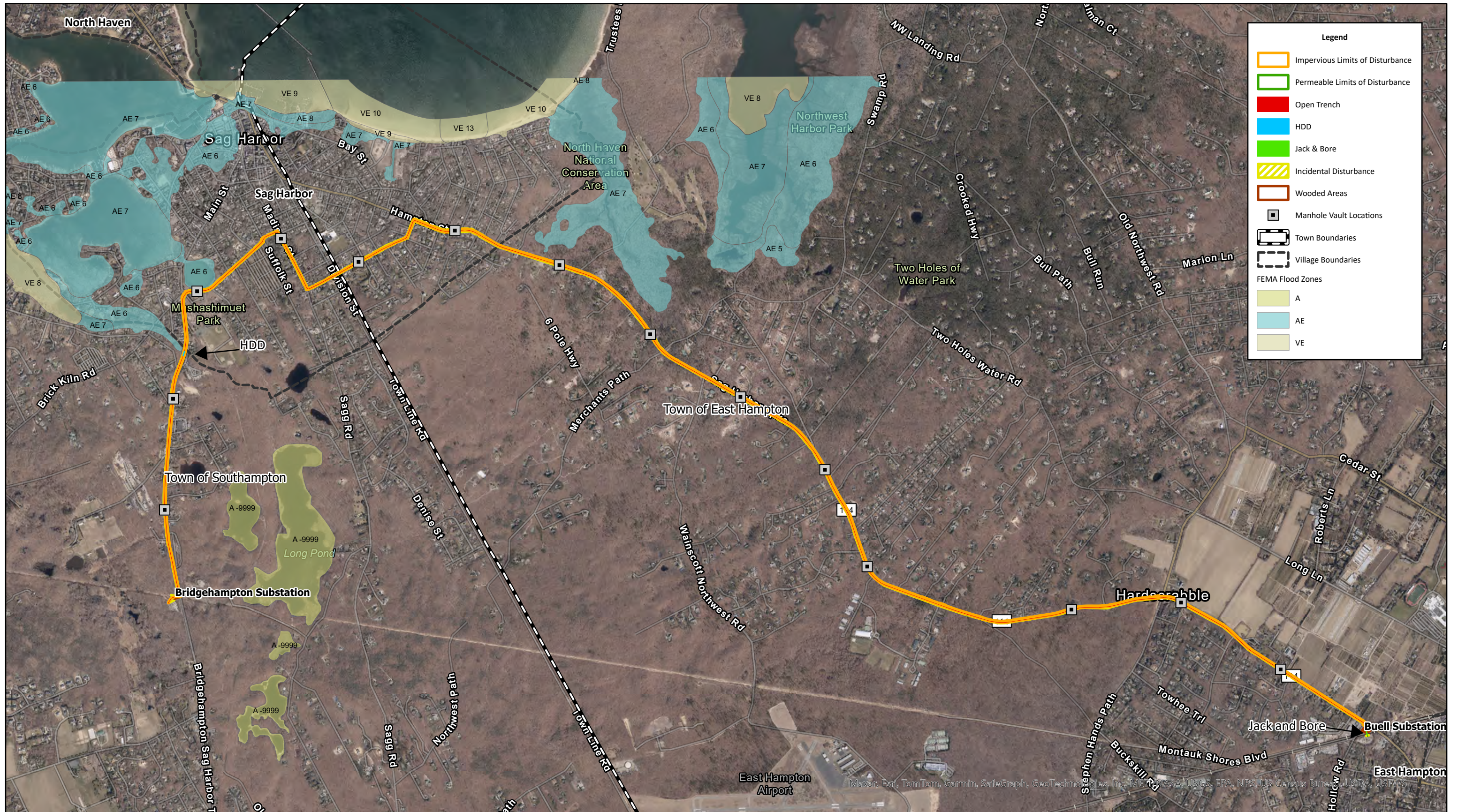
FIGURE 6 FEDERAL EMERGENCY MANAGEMENT AREA (FEMA) FLOOD ZONE MAP BRIDGEHAMPTON TO BUELL NEW 69KV UNDERGROUND TRANSMISSION CABLE
