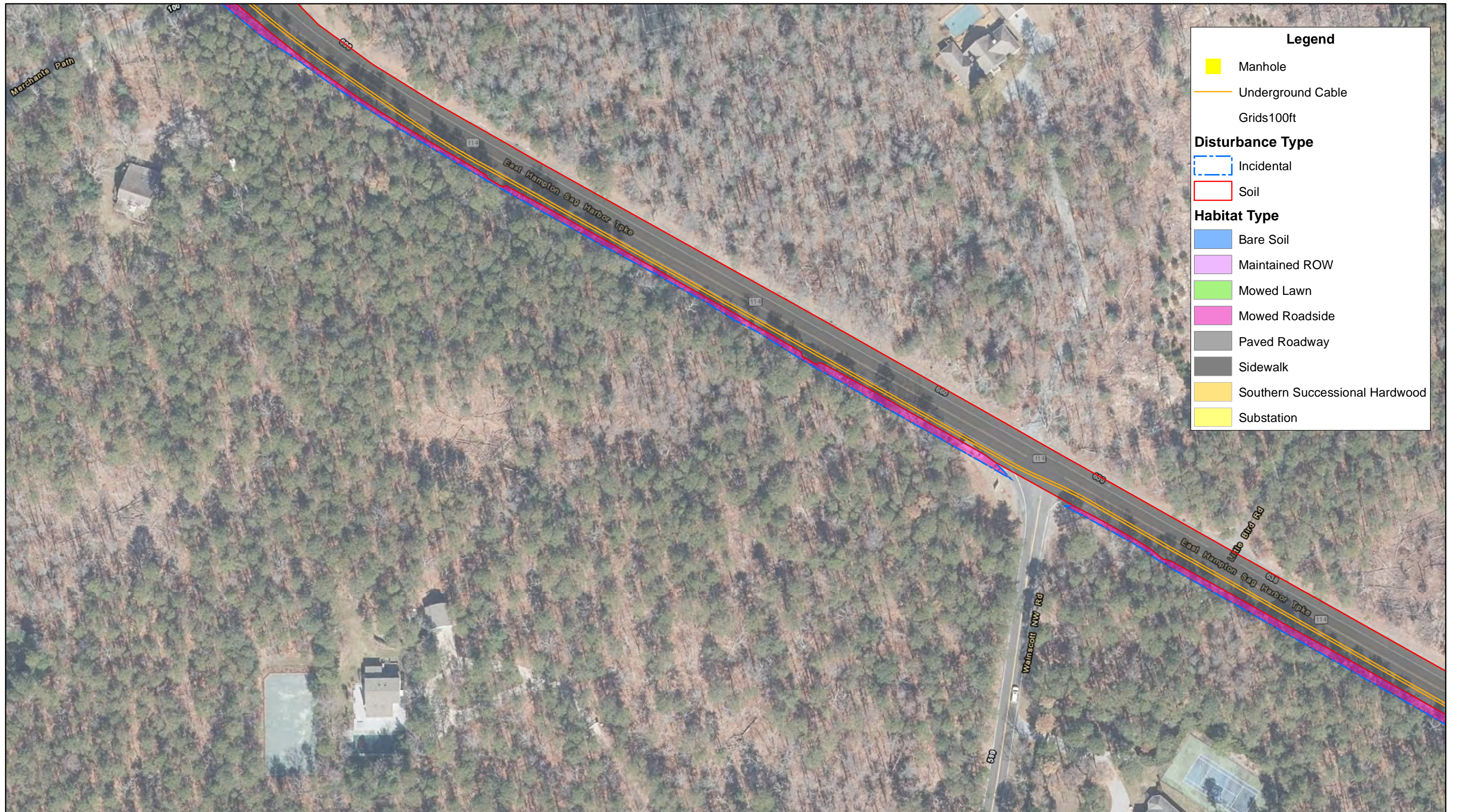
FIGURE 9-18 PREFERRED ALTERNATIVE HABITAT MAP BRIDGEHAMPTON TO BUELL NEW 69KV UNDERGROUND TRANSMISSION CABLE
