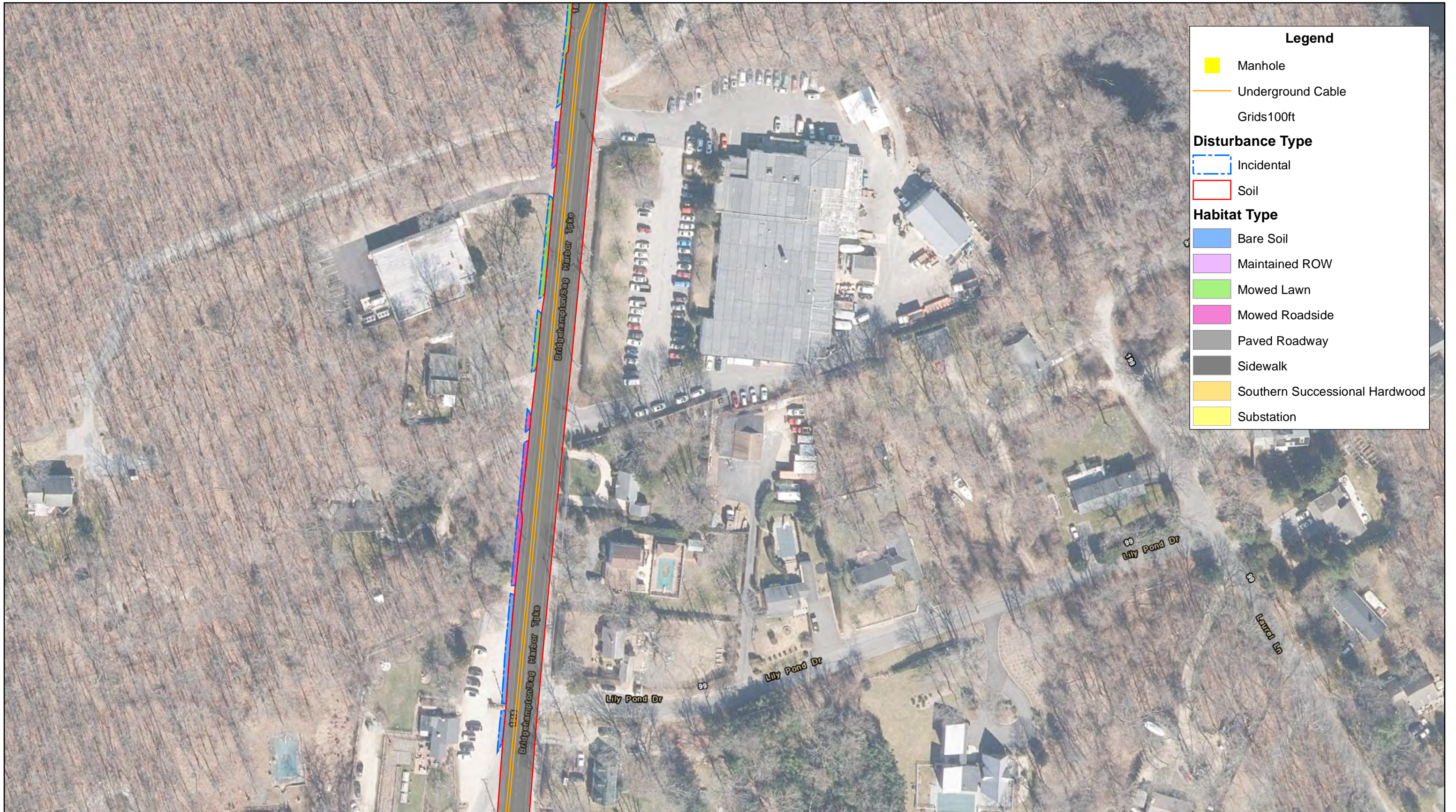
FIGURE 9-5 PREFERRED ALTERNATIVE HABITAT MAP BRIDGEHAMPTON TO BUELL NEW 69KV UNDERGROUND TRANSMISSION CABLE
